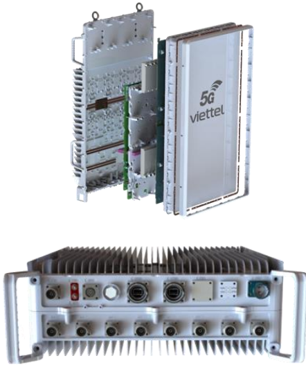
Figure 2. Viettel 5G Massive MIMO 8T8R and 32T32R transceiver stations (Operating frequency band 2496 – 2690 MHz (FR1-N41-3GPP))
