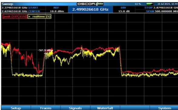
Figure 17. The results measured of the jammer in the 2500 MHz to 2690 MHz band on OSCOR Green
